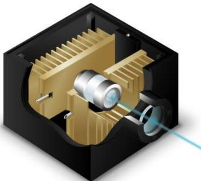
**Figure 1.** Schematic drawing of the Cermax arc lamp and lamp housing in ISS spectrofluorometers.
