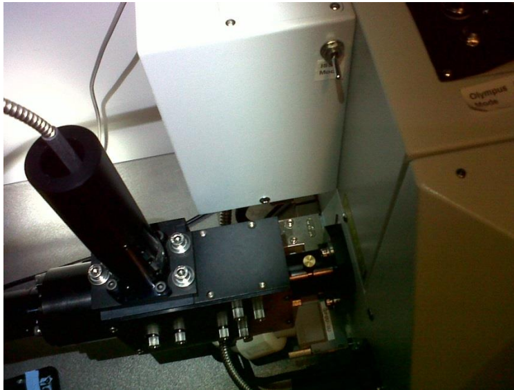
Figure 5.1 Laser combiner. The adapter from the Olympus laser launcher is connected to the left (point A); the adapter from the ISS laser launcher is connected to the top. The brass thumbscrew (C) allows for selection either laser launcher.
