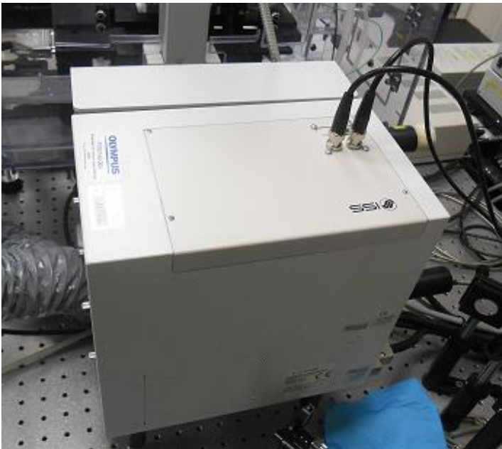
Figure 2.2 Confocal head of the FV1000 with the ISS panel for the Output signals of the internal detectors.
